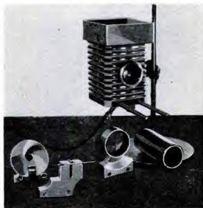
Above, completed lamp house with the top baffle being screwed in place, also the condensing-lens mount and the lamp fixture completed and ready for fitting in position. Below, the completed projector ready for use, with a gauging anvil for twist drills. Other anvils or holding fixtures can be made as required
